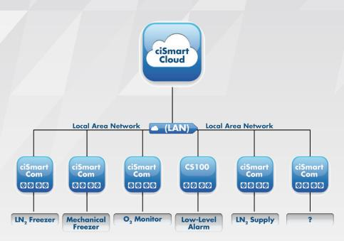
ciSmart™ Com is designed to extend the capability of liquid nitrogen refrigerators and freezers with monitoring, data collection, local and remote access, data graphing, alarm notification and advanced reporting.
