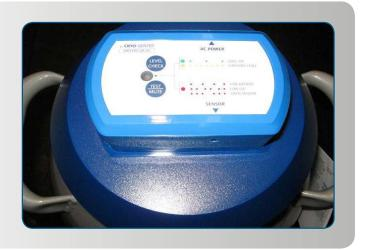
The Cryo-Sentry low level alarm is an optional accessory for selected models of portable liquid nitrogen refrigerators. It is designed to provide visual and audible alarms when the liquid nitrogen level drops below a preset level, usually 25 percent of the container capacity. This monitoring system provides a high level of security, alerting the user to low nitrogen levels, and serves as a reminder for a scheduled refilling.
