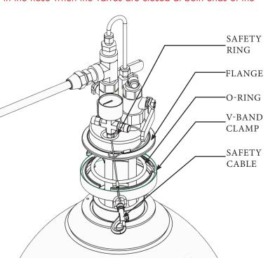
hose. If liquid nitrogen is trapped between the valves of the liquid cylinder and the LWD, it has no escape path as it warms and expands. The resulting pressure can cause the hose to rupture and may cause personal injury. The current model LWD is equipped with a pressure relief valve. Previous versions of the LWD must be used with a transfer hose equipped with a pressure relief valve.
