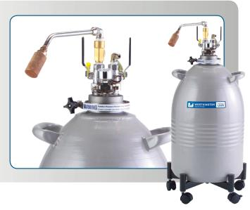
The Liquid Withdrawal Device (LWD) provides convenient pressure transfers of liquid nitrogen from 25LD, 35LD and 50LD Dewars. The device clamps directly to the special neck flange that is found under the plastic trim collar around the neck of these containers.
